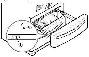
**4.** With the drawer pulled out to full extension, insert the drawer and Ice Bin in the rail assembly.
